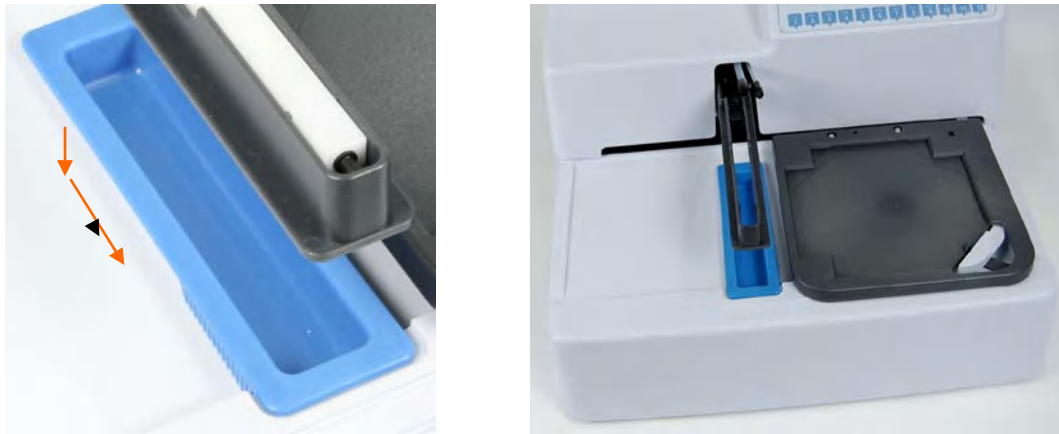
Figure 7. Priming vessel installation
