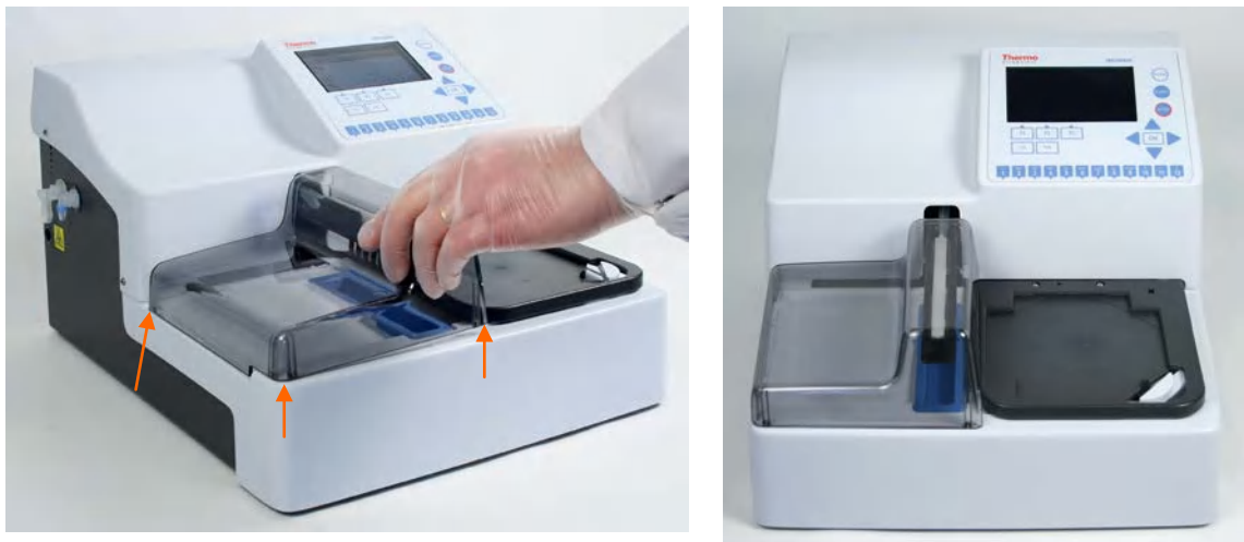
Figure 20. Installing the aerosol cover
