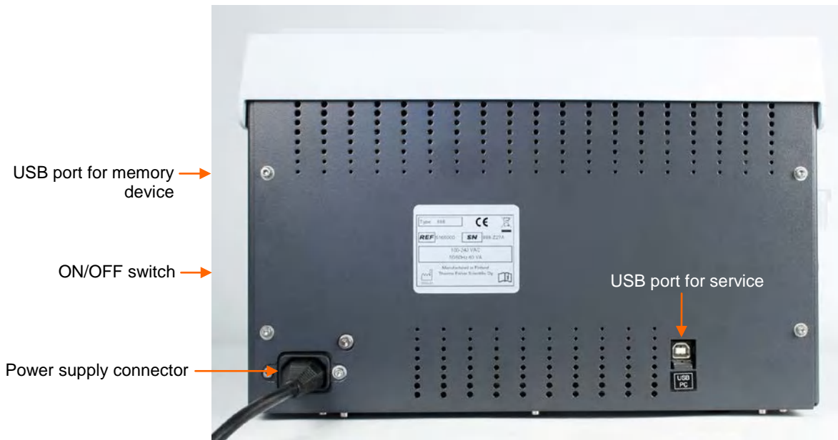
Figure 22. Wellwash back view
