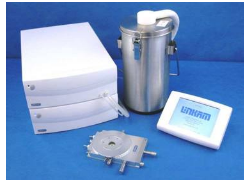
Cryobiology System including LNP95 liquid nitrogen cooling system
