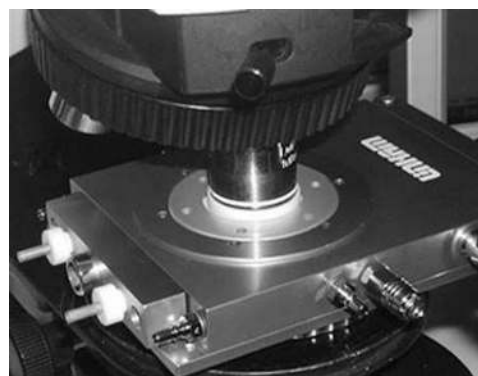
Diagram shows objective lens passing through the stage lid.
