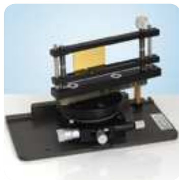
Dedicated PM-IRRAS sample holder for variable angle of incidence with different sample sizes.
