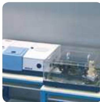
PMA50XL module for measurements with enlarged range for angles of incidence between 32.5° - 89°
