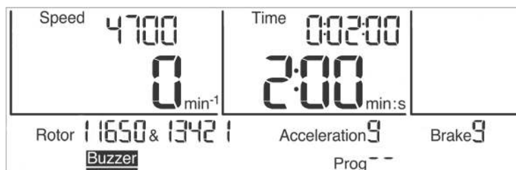
Fig. 20: The sound signal "Buzzer" is activated
