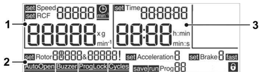
Fig. 11: Display of the "Spincontrol L" control system
