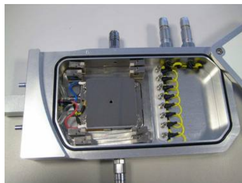
The LTS120E-PL8 Peltier heated/cooled probe stage with temperature range of -40^{\circ}\text{C} to +120^{\circ}\text{C} , fitted with spring post connectors and LEMO feed-throughs.
