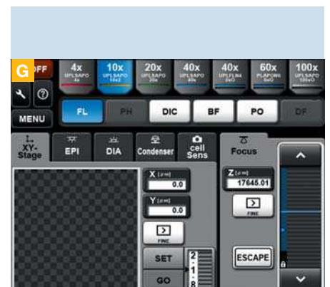
Full microscope control via touch panel user interface
