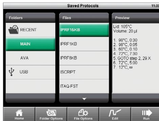
Fig. 6. Saved Protocols screen showing the preinstalled library of standard protocols in the MAIN folder.
