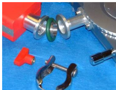
Pirani Vacuum gauge connections with THMS350V stage
