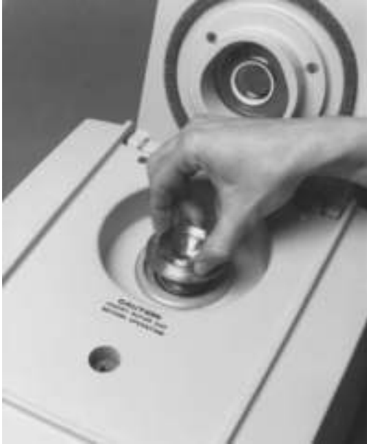
Figure 5.2 Lifting Out the Stator. Keep the stator level to prevent binding.
