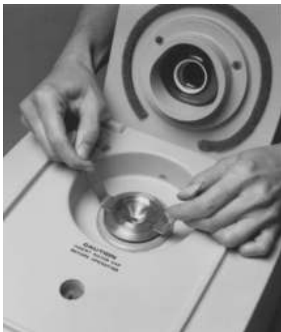
Figure 5.1 Prying Up the Stator
