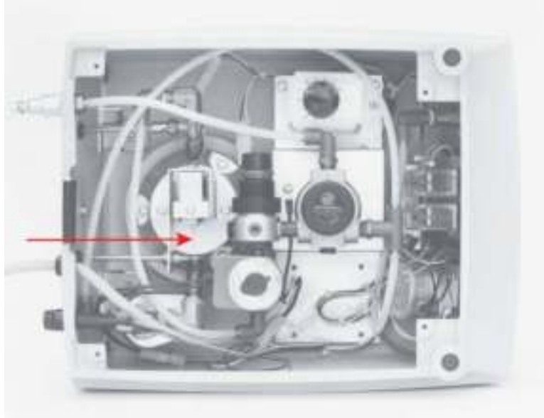
Figure 5.5 Location of the Brake Spring Wire from the Ultracentrifuge Bottom
