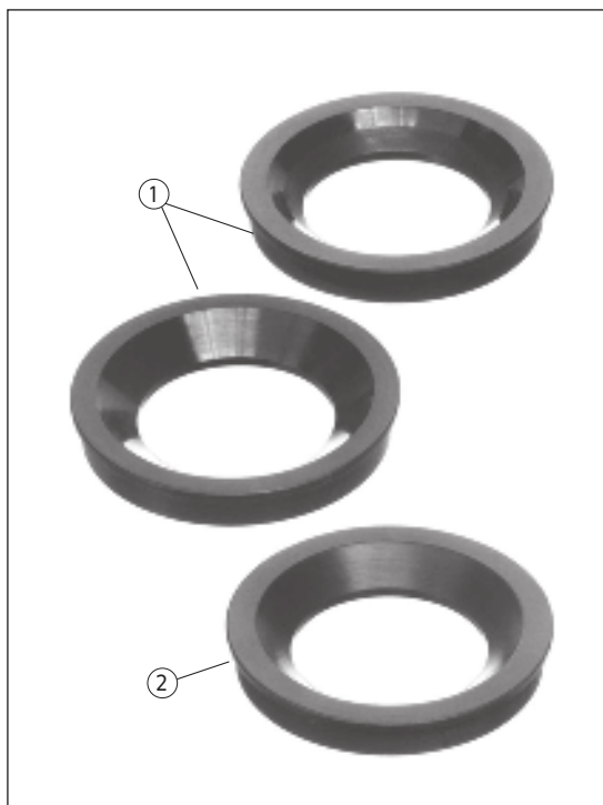
1. Worn Stator Pads 2. New Stator Pads
