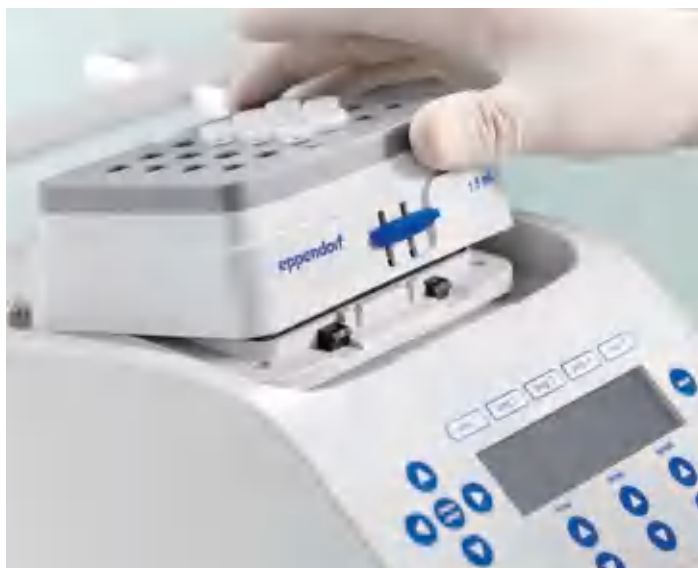
SmartBlock removal from Eppendorf ThermoMixer® C
