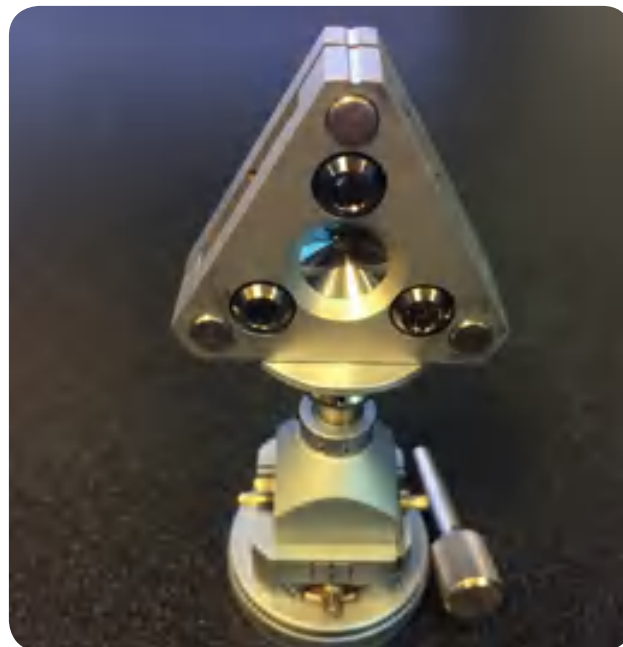
Figure 2: Bragg-Mini, a Merrill-Bassett DAC from Almax easyLab Inc.
