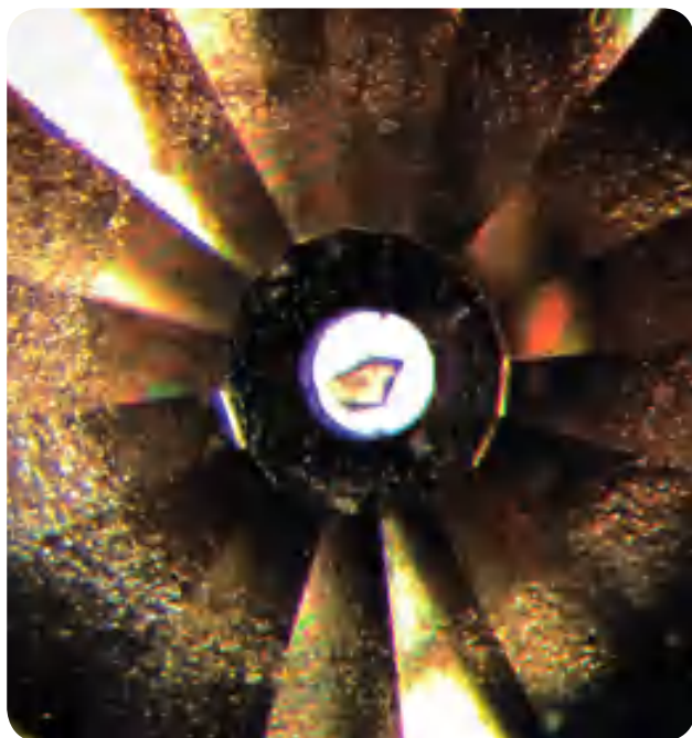
Figure 3: Small ylid sample mounted in the DAC
