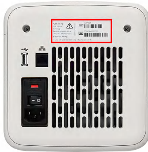
Figure 2 Location of the safety label on the rear panel of the instrument
