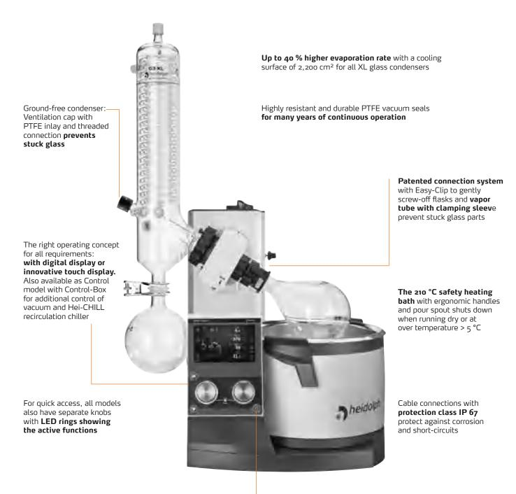
**For unlimited evaporation:** In conjunction with the Distimatic automatic module, you can distill indefinitely and automatically in 24 / 7 operation. The affordable alternative to large rotary evaporators.
