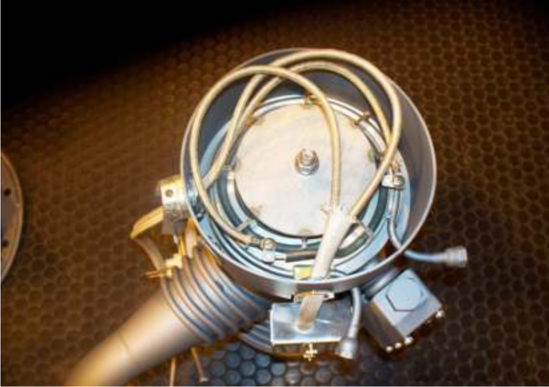
Figure 3-8 VHS-4 Heater Mounting
