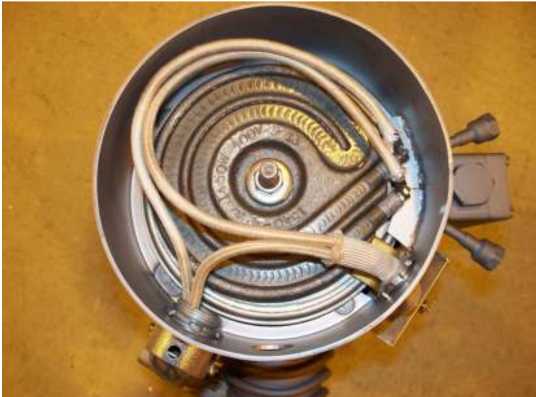
Figure 3-9 VHS-4, VHS-6 and VHS-250 with Platen Heater - Orientation of Heater (VHS-4 Shown)
