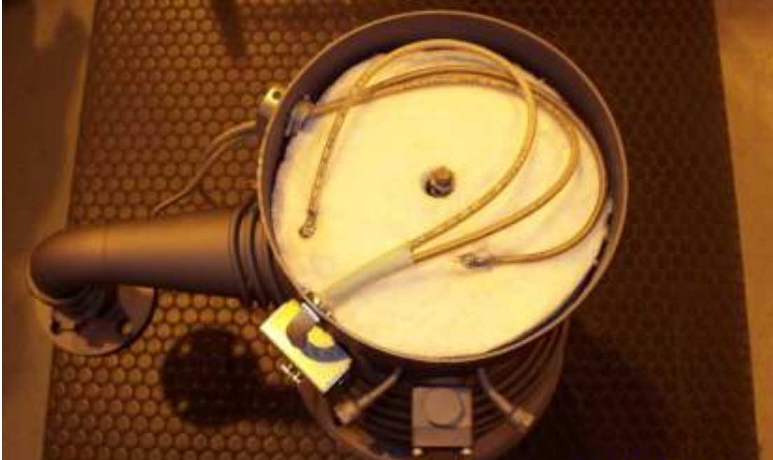
Figure 3-10 VHS-4, VHS-6 and VHS-250 with Tubular Heater Insulation and Wire Placement
