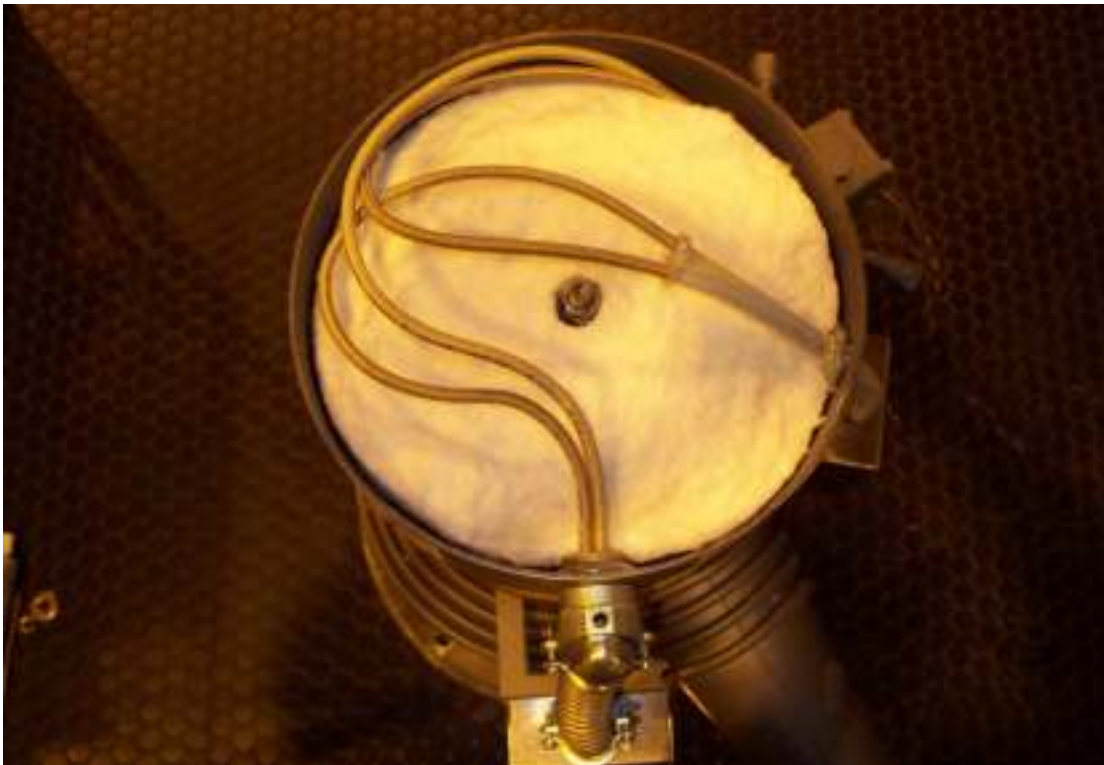
Figure 3-11 VHS-4, VHS-6 and VHS-250 with Platen Heater Insulation and Wire Placement
