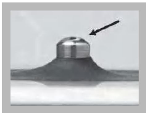
Unconditioned pedestal (droplet flattens out)
