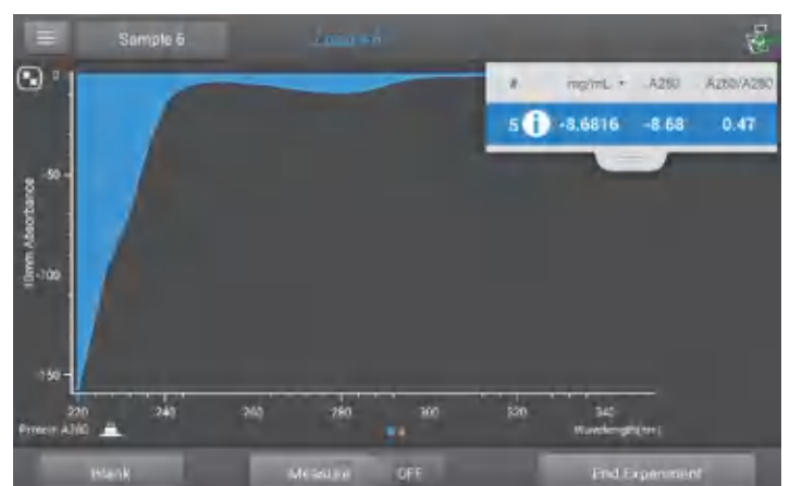
Protein sample solution used to blank instrument results in “mirror image” spectrum
