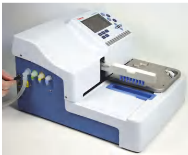
Figure 2–19. Connecting the liquid sensor cable
