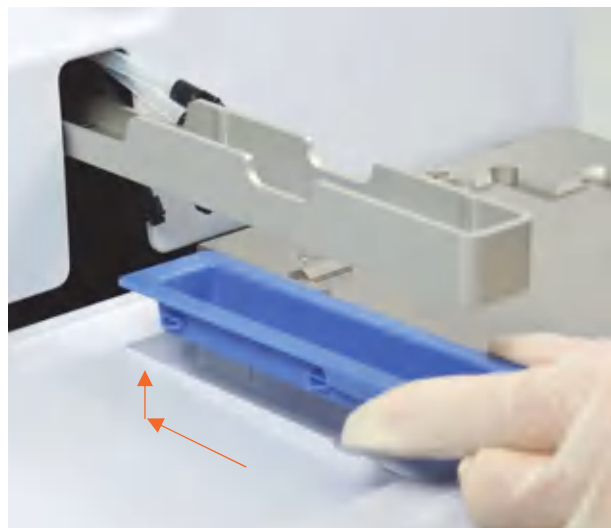
Figure 11–42. Removing the priming vessel
