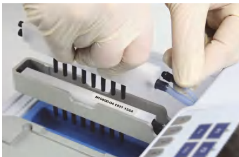
Figure 2–10. Fitting the wash heads to the connectors
