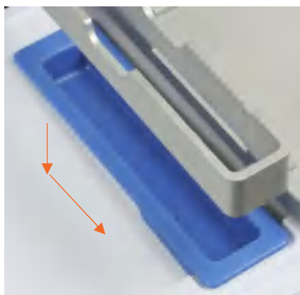
Figure 2–8. Priming vessel installation
