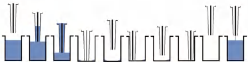
Figure 1–4. Principle of washing step (Sweep2)
