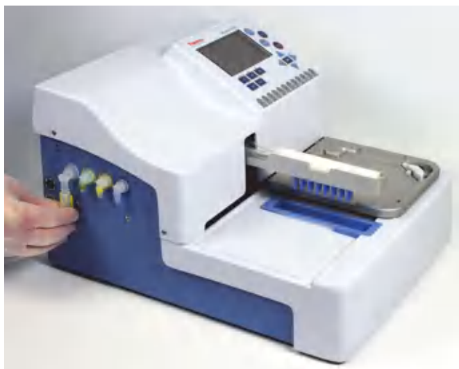
Figure 2–18. Connecting the liquid bottle tubing
