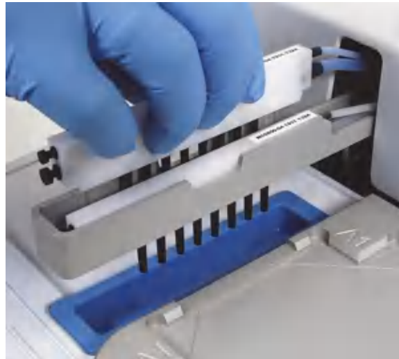
Figure 2–11. Fitting the 2x8 wash heads next to each other onto the wash head arm (A and B)
