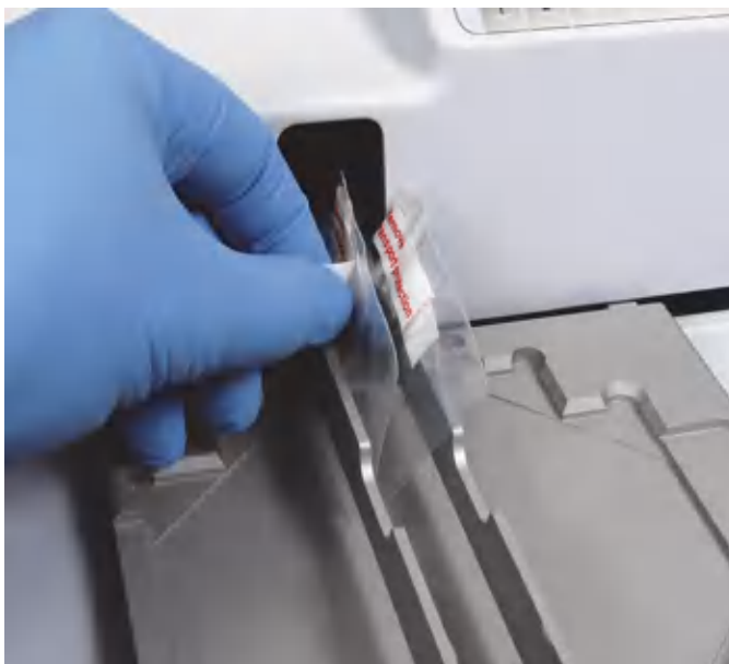
Figure 2–6. Transport lock and transport lock tag
