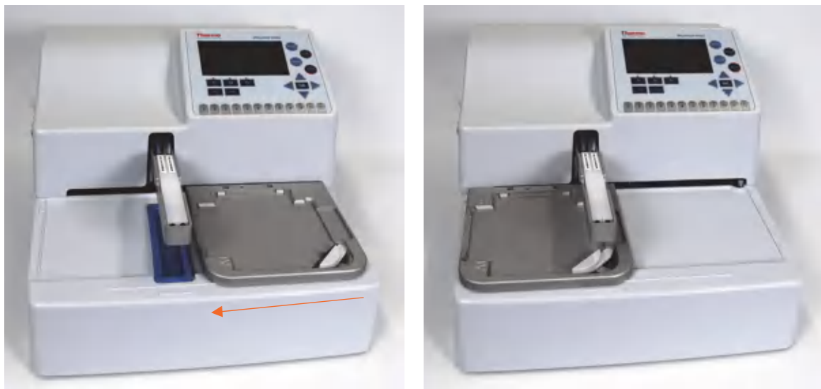
Figure 11–43. Cleaning the plate carrier and the surrounding area
