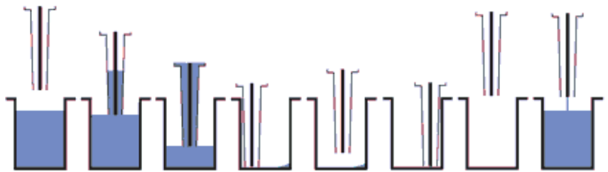
Figure 1–4. Principle of washing step (Sweep2)
