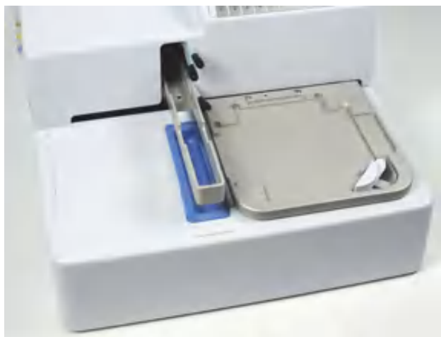
Figure 11–47. Aligning the plate carrier and wash head arm
