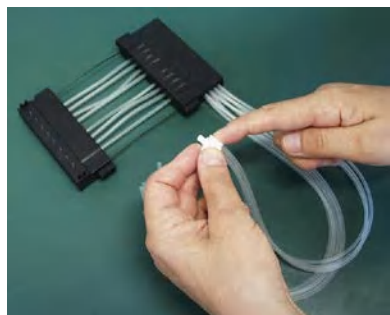
Figure 5-48. Inserting the tubes into the PEEK tubing weight
