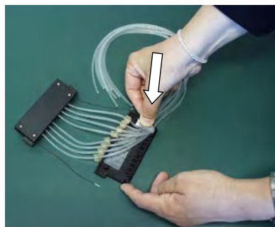
Figure 5–36. Pressing the tubing identification plate into place
