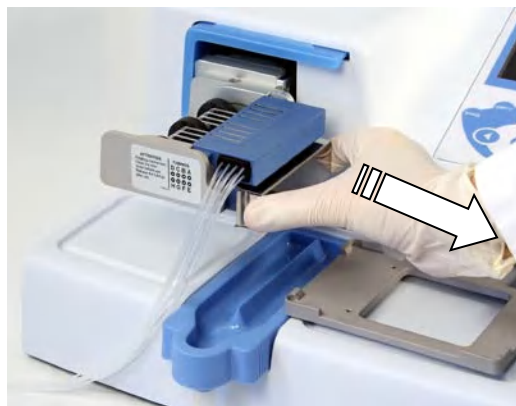
Figure 4–16. Pulling the tip protection off from the dispensing cassette
