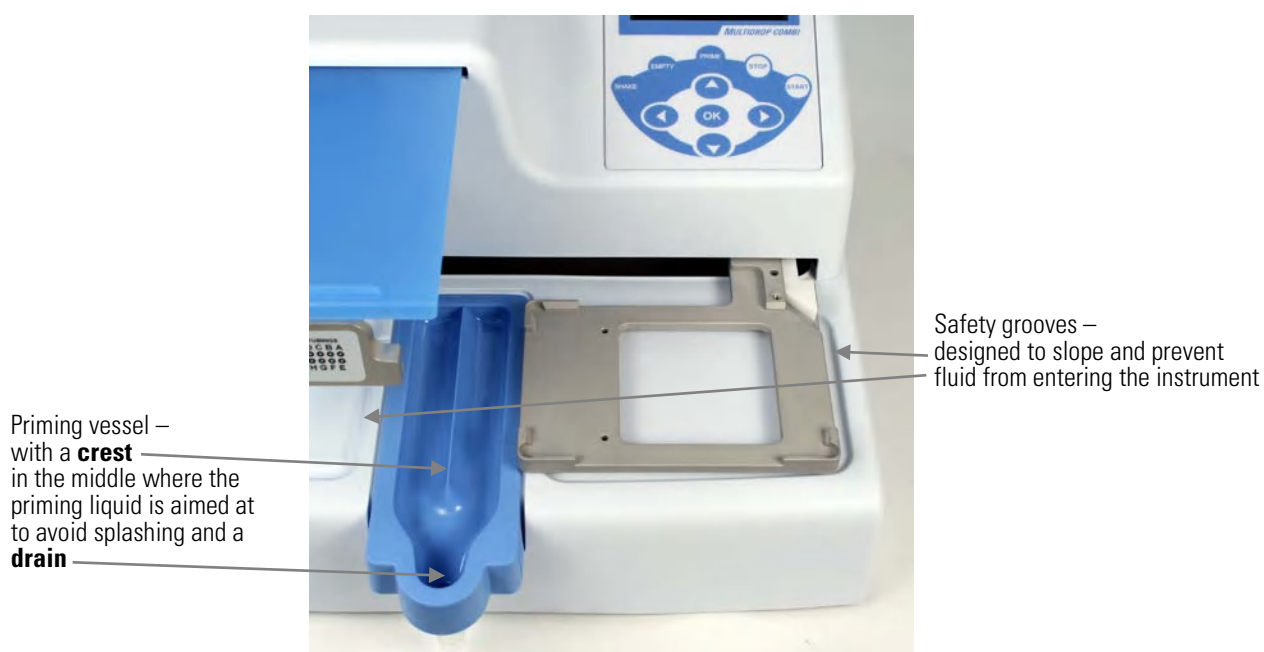
Figure 4–9. Priming vessel inserted into place
