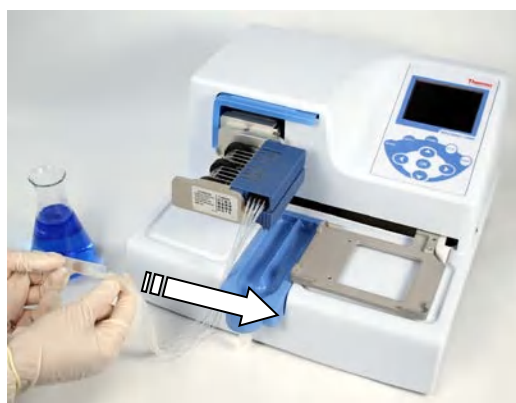
Figure 4–17. Removing the tubing weight protection and rubber holder
