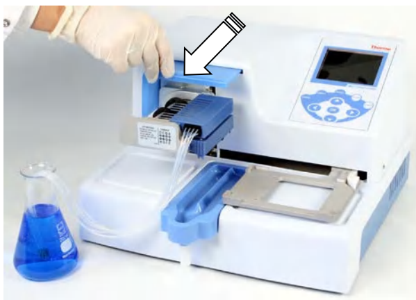
Figure 4–20. Pulling the rotor cover over the rotor
