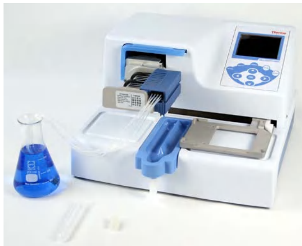
Figure 4–18. Cassette with the tip and tubing weight protections removed
