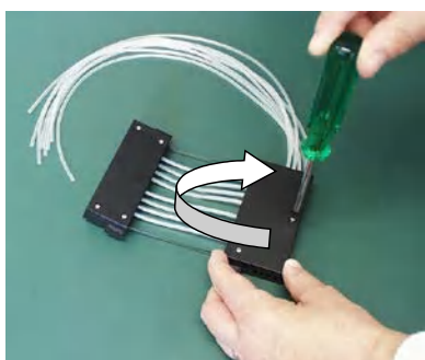
Figure 5-42. Fastening the cover retaining screws
