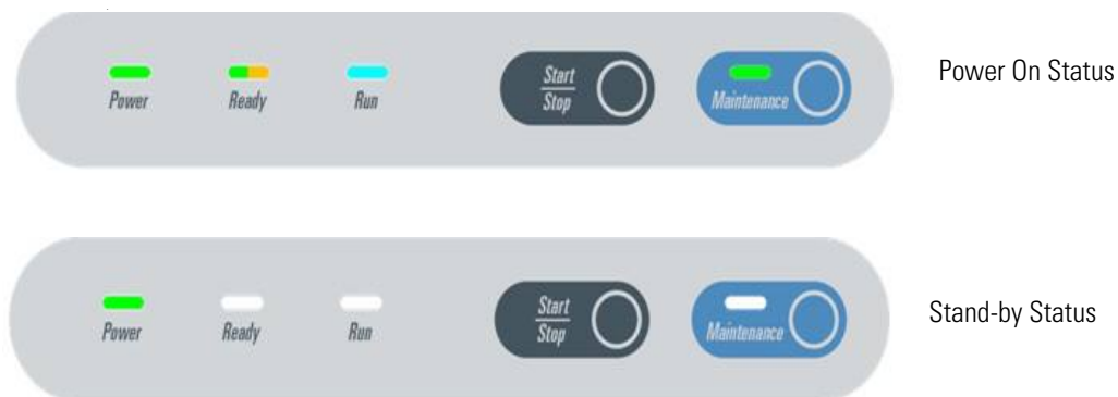
Figure 177. TRACE 1300 Status Panel at the GC Power On
