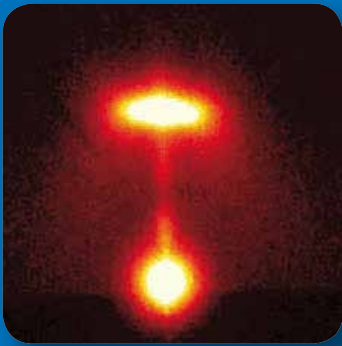
GISAXS pattern of an unaltered multilayer mirror
