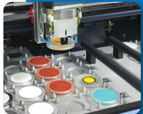
Loading tray with mechanical gripper
