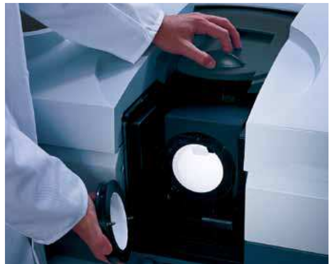
The diffuse reflectance accessory is ideal for measuring a wide range of solid and liquid samples.
