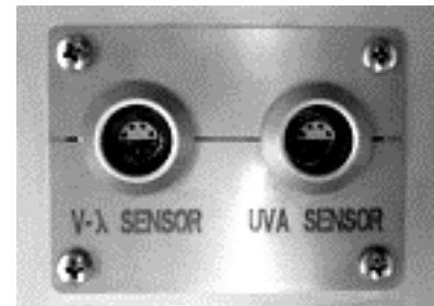
Figure 13: Lemo sockets to connect the light sensors
