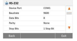
Select the following items to set RS232 port when RS232 port link to printer or other RS232 compatible device.
