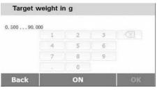
Enable the Target weight and press ON button.
