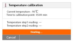
The dryer unit is heated to a temperature of 100°C. You can observe the progress on the display as the dryer temperature and count down period are displayed. After 15 minutes, read the thermometer through the inspection window on the cover and enter this temperature. Adjust the display reading to agree with the thermometer, then press the Enter button. You have 15 minutes to make this adjustment, otherwise the calibration is terminated.
