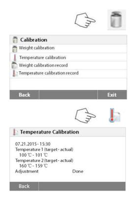
Press Weight and temperature calibration button to access the calibration screen. Press **Back** to return to previous screen. Press **Exit** to return to Home screen. Press the Temperature calibration history button.
