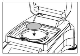
Place the empty sample pan and glass fiber pan in the pan handler. The sample pan must lie flat in the pan handler.
