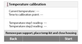
You are now prompted to remove the pan support. Place a temperature calibration unit and close the upper housing.
