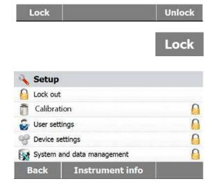
Press **Lock** to lock out Press **Unlock** to release.
