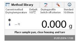
To switch the Moisture Analyzer on, press the On/Off button. An internal diagnostic test is performed; the display lights and the Home screen appears followed by the initial display.
