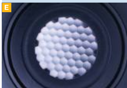
E Fly-eye lens for homogeneous fluorescence illumination
