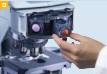
Easy replacement of filter cubes
