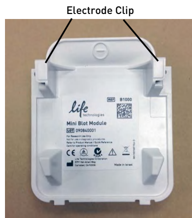
Cathode core, exterior
