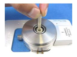
Once the sample holder is positioned in the heater assembly place a fore finger on top of the sample holder. Gently press down and rotate the sample holder so that it sits firmly in place.
