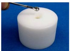
Load Sample Holder into CCR1000 Carefully pick up the top of the Sample Holder and hold it over the heater assembly.
