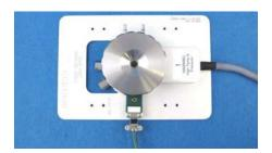
Make sure the '+' and '-' markings on the cable and connector match and push the cable firmly in place.
