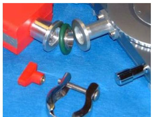
Pirani Vacuum gauge connections with FDCS196 stage
