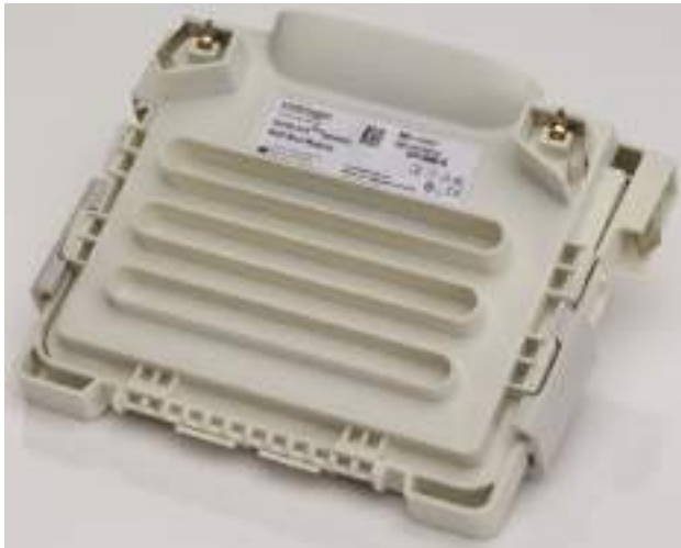
Figure 3 Cathode core exterior of Blot Module.
