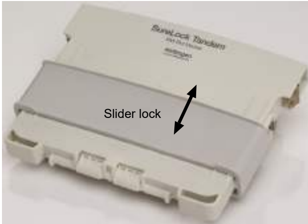
Figure 2 Blot Module showing anode core exterior and slider lock.
