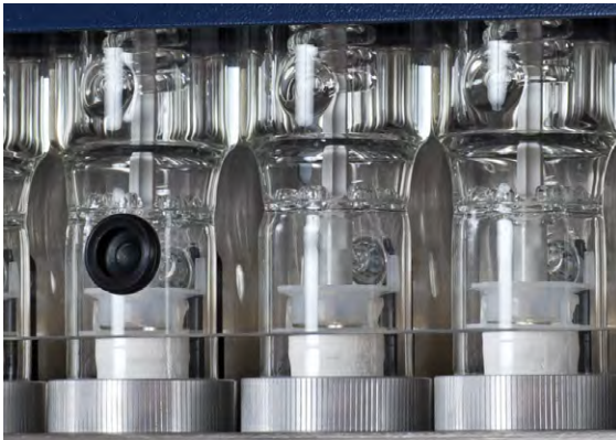
Built-in fume hoods prevent exposure to solvent fumes during addition of solvents.
