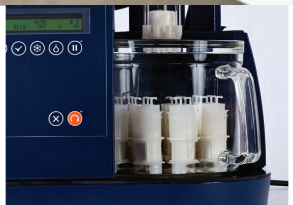
12-place hydrolysis sample holder for unattended operation and higher throughput.
