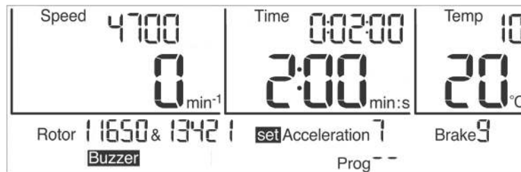
Fig. 20: Preselection of a curve; here: preselection of an acceleration curve
