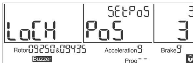
Fig. 29: Indication after the completion of the positioning process
