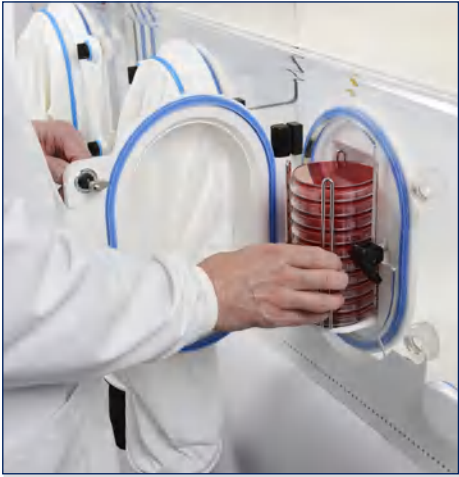
Insert 10 Plates through the glove port
